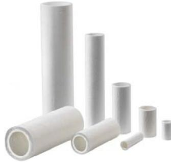
**Our Microfiber disposable filter elements** are manufactured from precise mixtures of borosilicate glass microfibers to the very highest standards. These elements offer exceptional filtration efficiency at very low-pressure drops and being +90% void volume give very long service life.
