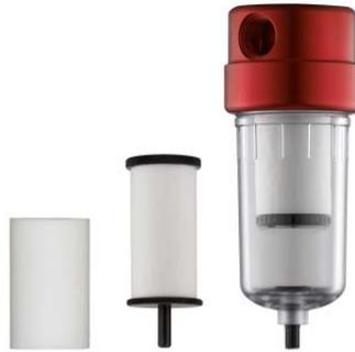
Our high efficiency PEL filter elements are constructed from virgin polyethylene (H.D.P.E.). The material is in powdered/granular form and then compressed into a sintered tube. This process allows the filter element to be free from foreign binders. Thus, the only compatibility issue is with polyethylene. No end caps or gaskets are necessary to seal the element into place. Axial compression is used to create a seal on the flat surface of the element. The PEL elements are naturally hydrophobic.
