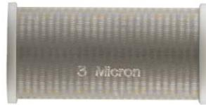
**Stainless Steel** elements are recommended for filtration of heavily contaminated gases, liquids, polymers, and steam, since they are re-cleanable by back-flushing or ultrasonic cleaning. The elements consist of five layers of precision-woven 316L stainless steel mesh formed into cylinders and sintered together.
