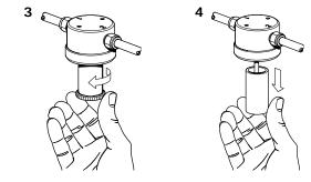
Disposable and sintered PTFE filter elements are sealed by compression against a flat surface. Gaskets are not required between the filter element and components of the housing. The stainless steel elements use a gasket at each end. The element is located by guides which fit the inside diameter of the tube at each end. In most housings the element is sealed by tightening a threaded element retainer.
